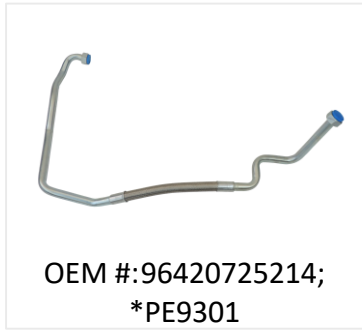
1989-1994 Porsche 911 964 Engine Oil Line (Connects Oil filter console to engine, not for Turbo Engine)
